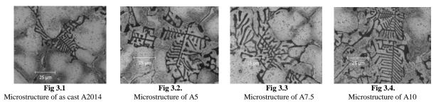
Figures 3.1 to 3.4 show the uniform distribution of ceramic reinforcement in A2014 matrix. The chinese script indicates the intermetallic compound of Aluminium with Cu, Si and Mn.
