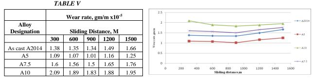
Fig 3.8: Wear rate of A2014 and its alloys
